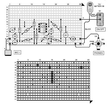
Fig.2. Stripboard component layout, off-board hard wiring, and underside view showing breaks required in the copper tracks.
