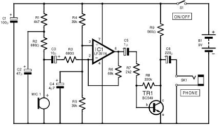
Fig.1. Complete circuit diagram for the Acoustic Probe.
